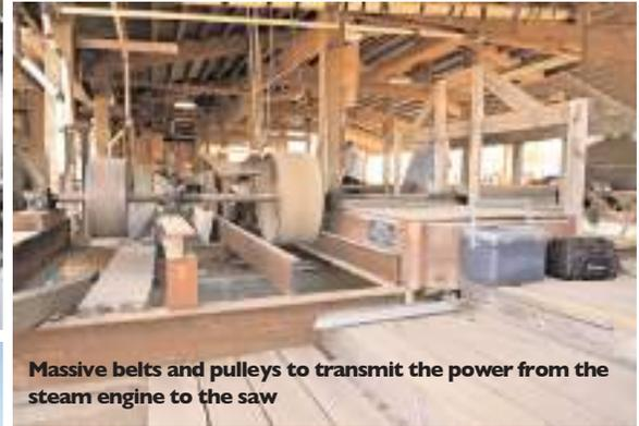
Massive belts and pulleys to transmit the power from the steam engine to the saw
