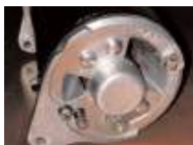
Example of C.E. bracket for 22462/D with Lucas script
