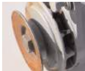
Early C45PVS integrated pulley and fan as one casting (C1076)
