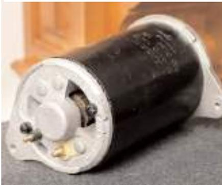
C45PVS-5.) Most parts remained the same, apart from a new armature (now part number 239511), a new commutator end-bracket (now 54210072) and brushes with their springs (54210090 and 54210091 respectively). Output is now 25 Amps. The C45PVS-6 was used on the later XK 150s and on the 3.4 and 3.8 Mk II saloons in the 22496D version (not USA & Canada for which markets the C48 model was used.)
