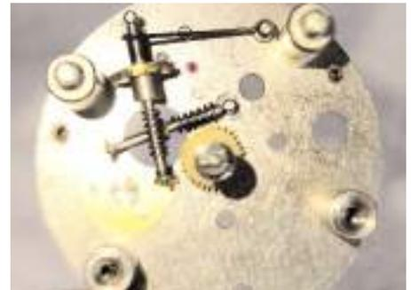
**View of gears clearly showing jeweled bearing for balance wheel assembly.**
