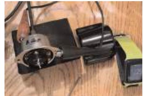
Reassembled clock showing speed adjustment on the bench. Note alligator clips with power directly from the car battery.
