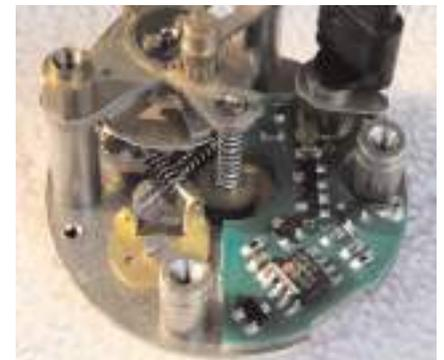
**Reassembled clock with PCB board installed, replacing faulty contacts mechanism. Note that the solenoid is not shown; its reinstallation is the final task.**
